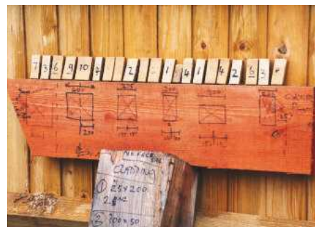
Carpenter Oak's clever lottery system for fixing ensures that no two panels are identical
